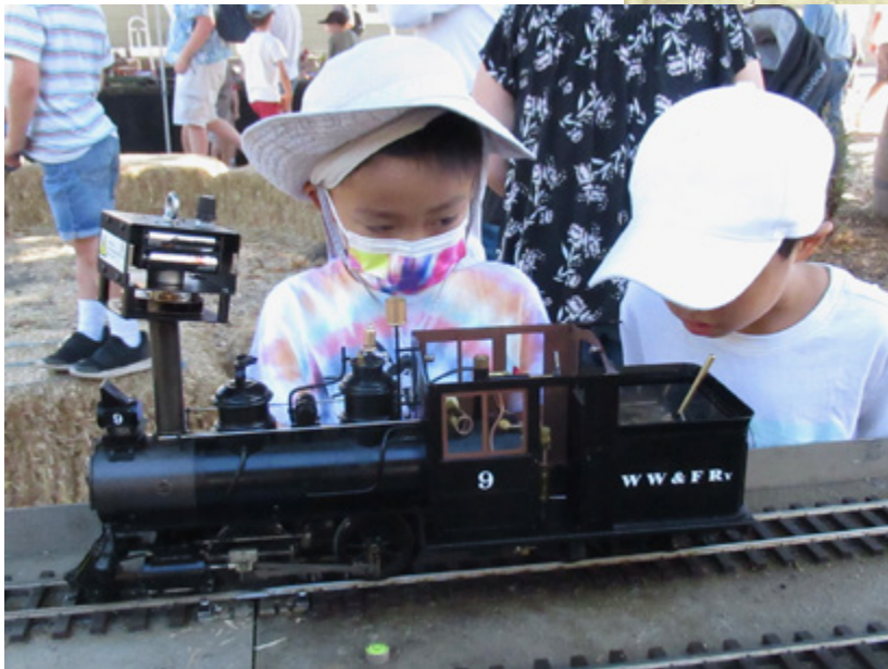
Intense observers check out Tim Boles' 7/8 Accucraft Forney. Note the fan on the chimney stack even though the engine burns butane.
