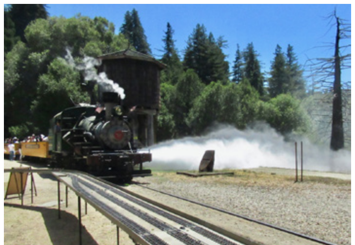
An uncommon sight: A blow down by the water tank.
