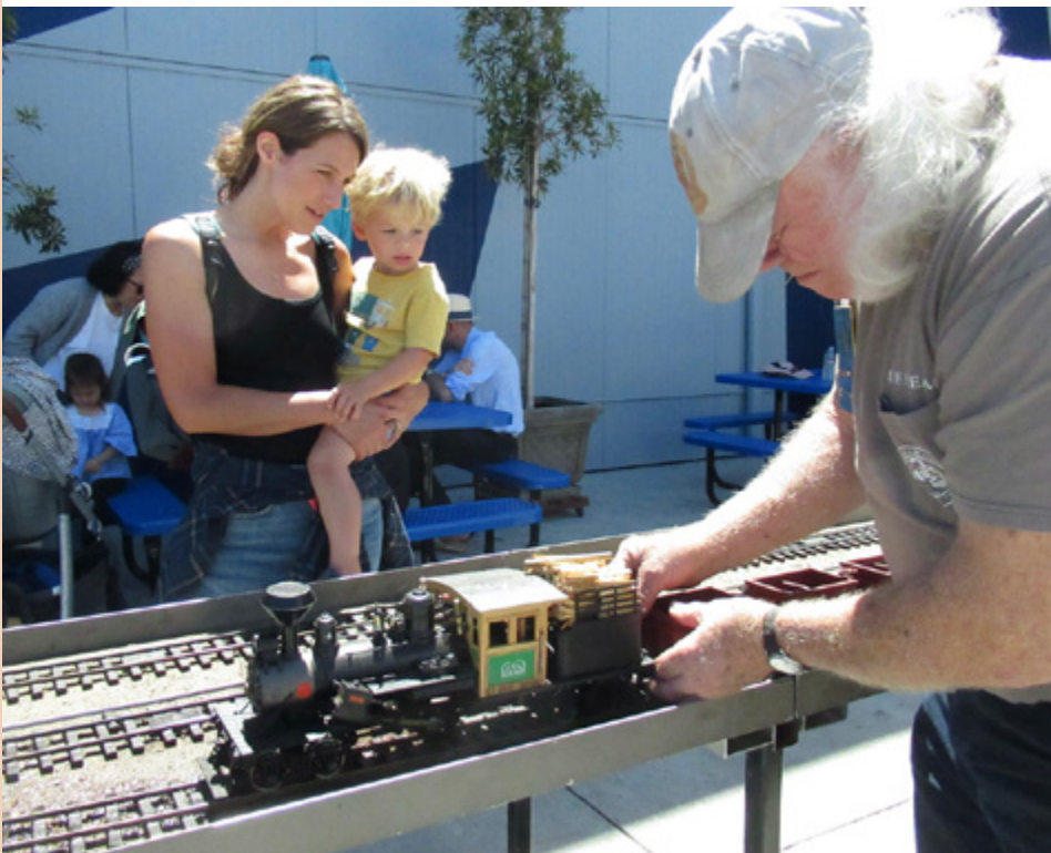
Gary Whaley finishes connecting a hook and loop couple on his Heisler.
