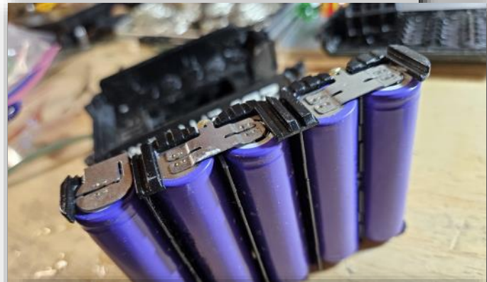
Five 18650 Li-Ion cells in series is 18.5 Volts
