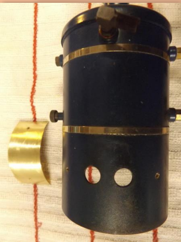
Photo to the left shows the two \frac{5}{64} " holes drilled into the boiler and the rounded brass plate to be mounted inside of the boiler
