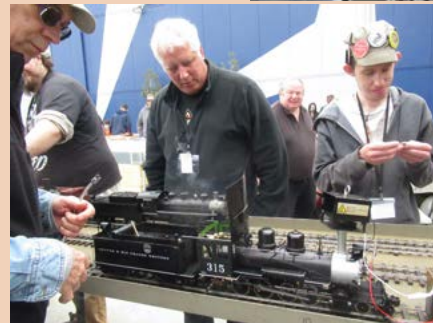
Lewis Breon (far left) is supervising the preparation of new BAGRS member (in the middle) Brian Parry's Accucraft C-18. Because the engine has a ceramic burner, it needs the fan on top of the chimney to create a draft despite being a butane fired engine. New BAGRS member Colton Snell is on the right.
