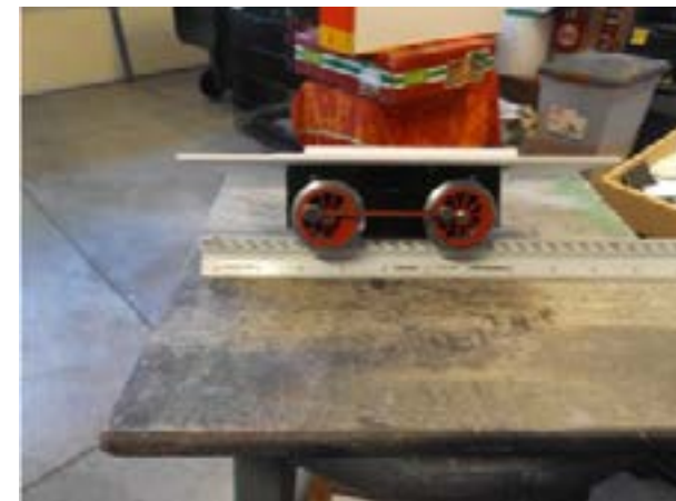
Motor block installed
