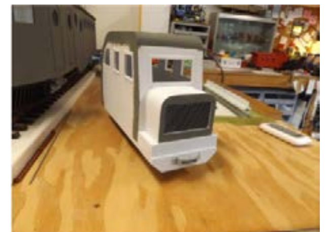
Windows trimmed and engine cowling in place
