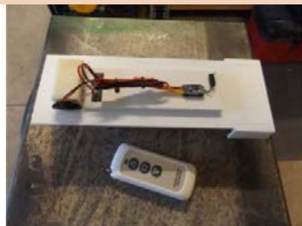
R/C control board wired to motor and battery
