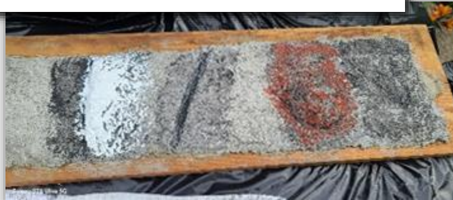
Using various techniques such as wrinkled aluminum foil on the wet stucco and choosing the appropriate stain colors
