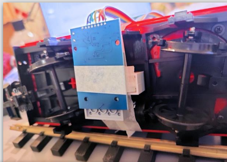
Measurement car with RC522 card reader, mounted approximately 3 mm (0.118 in.) from the track
