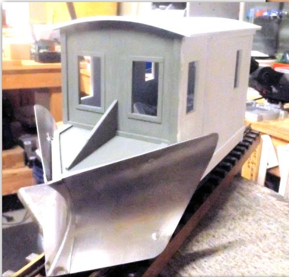
Here's the front view of the snowplow, showing the covering and wedge that hides the mounting brackets.
