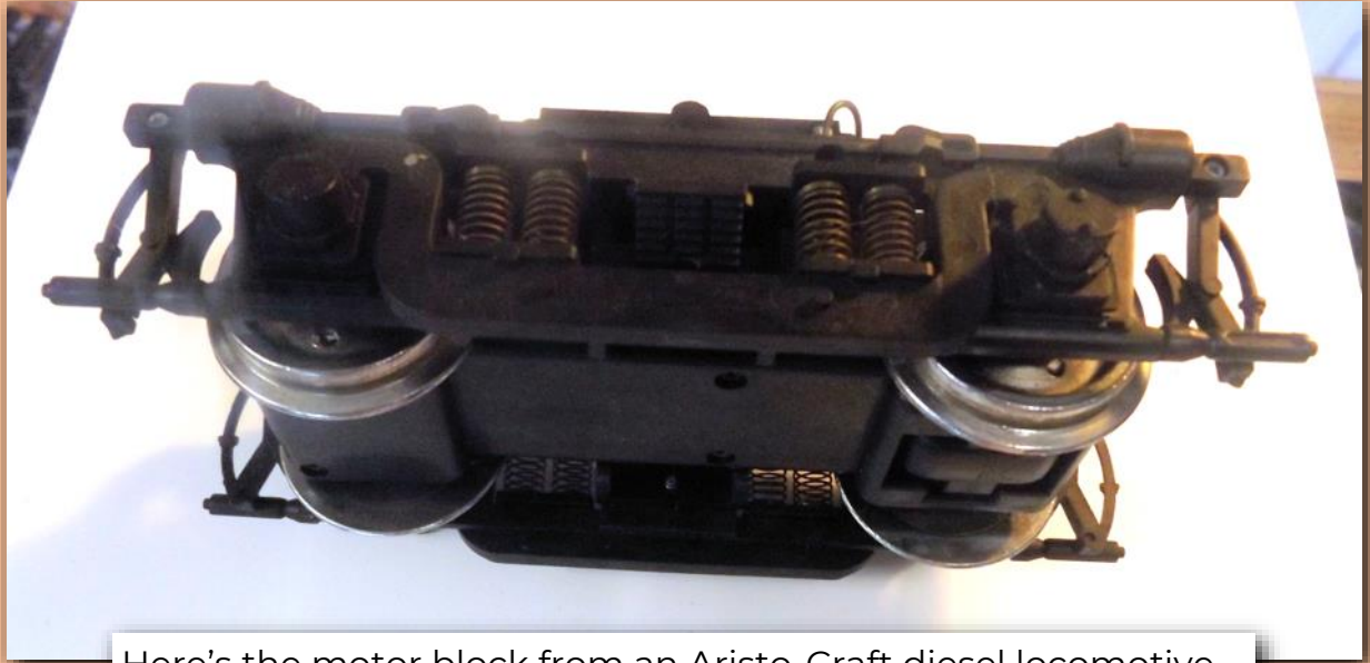
Here's the motor block from an Aristo-Craft diesel locomotive.
