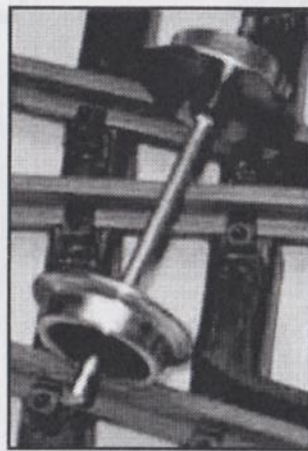
Figure 1a: Wheels on the curve are entering the frog area and guard rail simultaneously.
